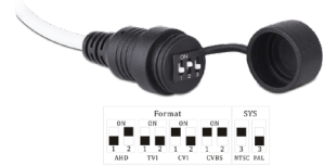
DIP Switch for Output Selection
